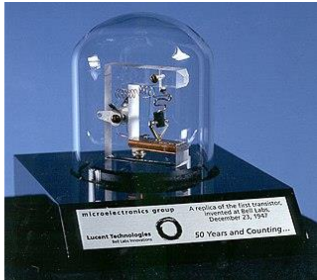
Fig. 4.12 Replica of the first working transistor
