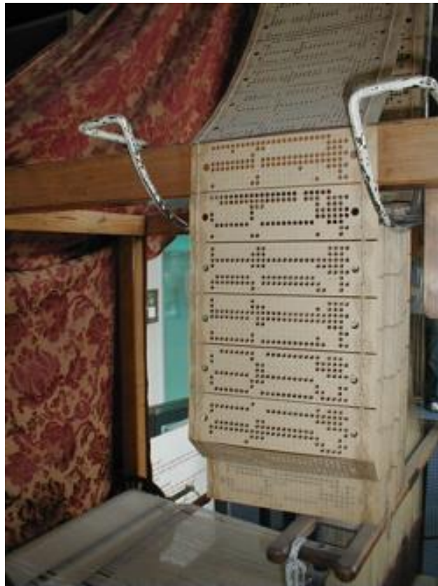
Fig. 2.5. Punched cards for loom templates 12
