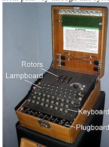
Fig. 2.18. Enigma rotor system 20
