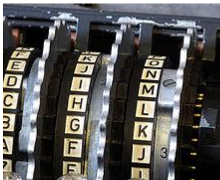
Fig. 2.18. Enigma rotor system 20
