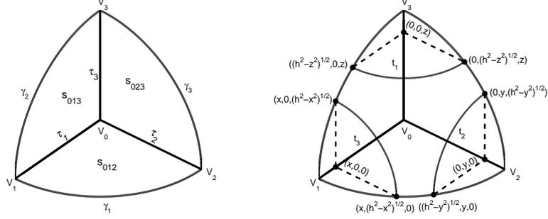
FIGURE 3. Tetrahedron with three curved edges
